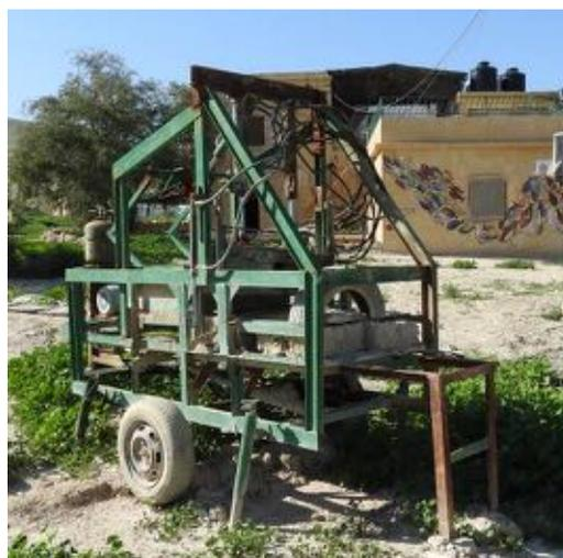
**Machine for making mud bricks**
